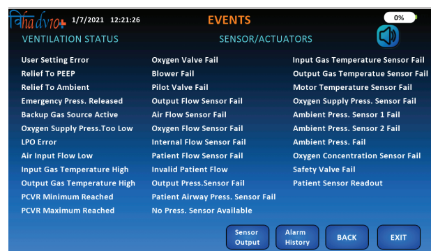
Display of all alarms, events, triggers with their respective status in Real Time. This gives the user complete understanding of all critical events and a protection against each safety event / malfunction.
