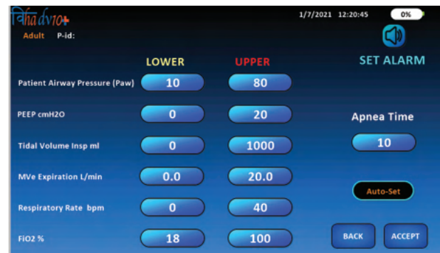
ALARM SETTING for monitored parameters with Auto-Set function
